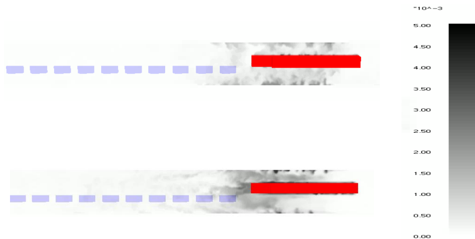
Figure 8: CO mass fraction as equivalent toxic 2 m above ground during the evacuation process for the standard curve (top) and adapted one (bottom) after 4 minutes
