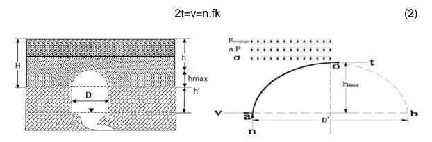
Figure 1. (a)Original karsts cave and equilibrium arc of the soil hole. Where hmax refers to the height of the pressure arch above the cave ceiling, which is the limit equilibrium height of a soil-hole arch; and H is the thickness of cover-layer soil (one layer or more) (He Keqiang et al, 2004). (b) Mechanical condition of the pressure arc (He Keqiang et al, 2004)
