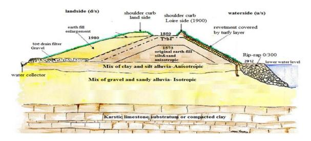
Figure 3.Typical cross section of a Loire levee nowadays (courtesy Jean Maurin) (International Levee Handbook, 2012)
