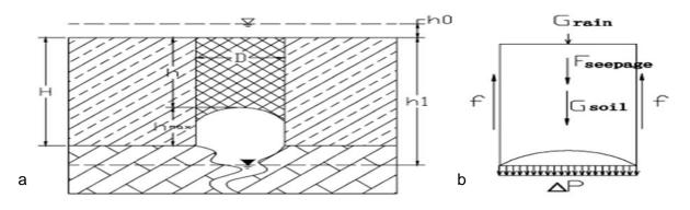
Figure 2. (a) Cross section of the karsts collapse column, (b) Mechanical analysis of the karsts collapse column (He Keqiang et al, 2004).
