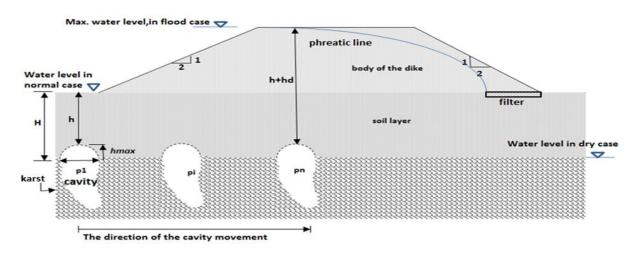
Figure 4. Different positions of sinkhole (horizontally from position p1 to position pn = 14 m)
