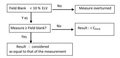
To compare the measurement result with the field blank value, the rule of calculation stated above in the case of analyses lower than the LoQ must be observed, whenever the results of the measurement are from the analysis of several compartments or only one (see example in the table hereafter).
