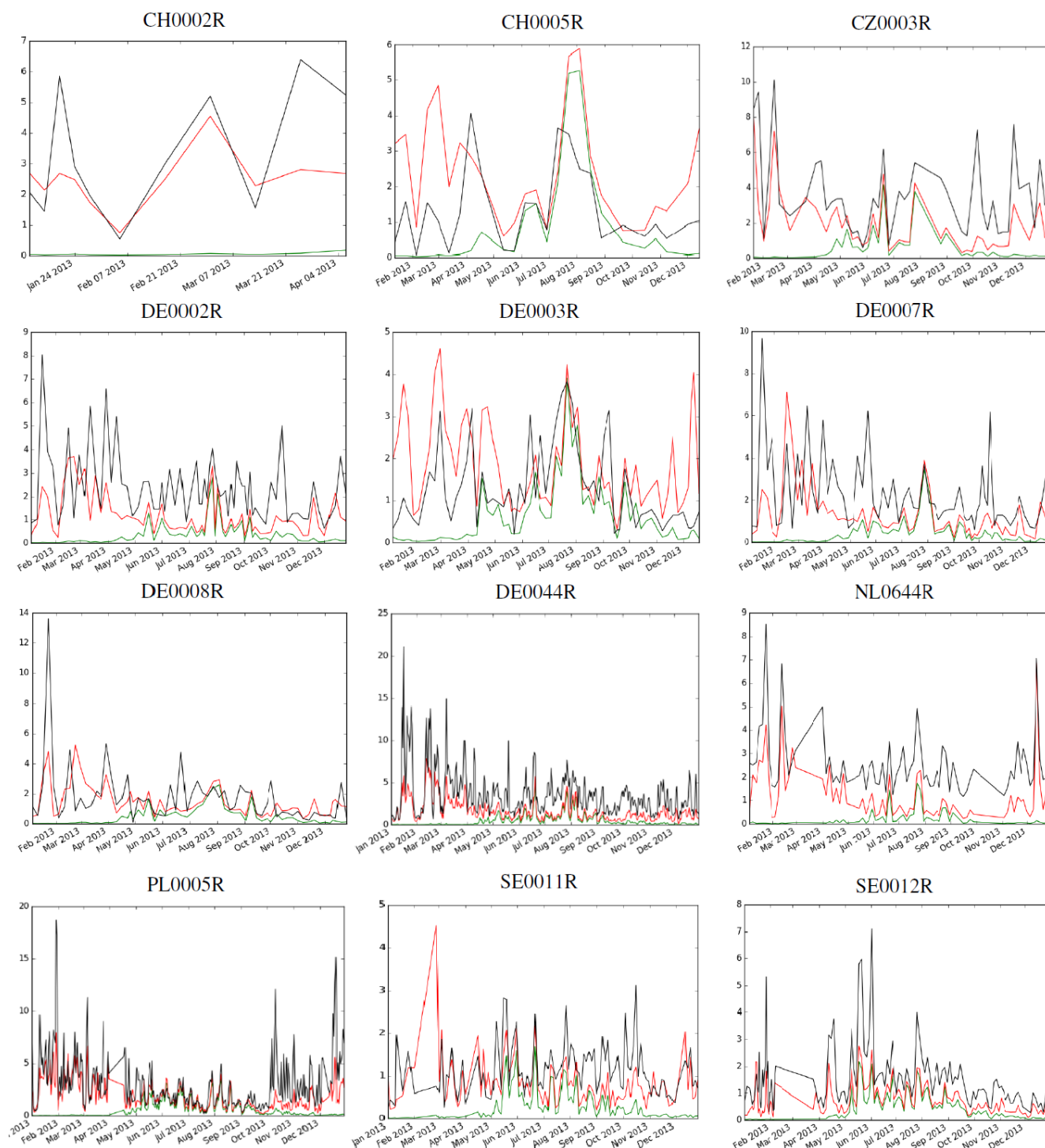
Figure 10. Temporal evolution of modeled (red line) and measured (black line) OC concentrations (in \mu\text{g m}^{-3} ) for stations in the south of Europe. The green line corresponds to OC from biogenic compounds.
