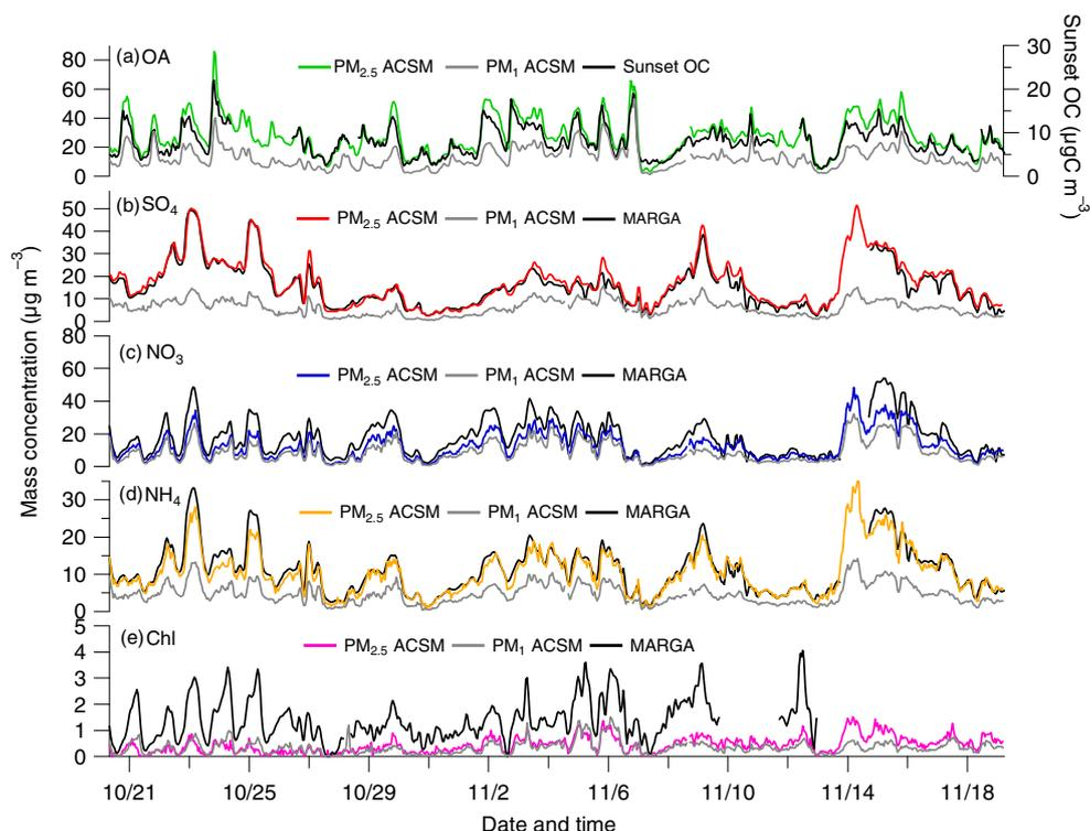
**Figure 2.** Intercomparisons between the NR-PM<sub>2.5</sub> mass concentrations measured by the PM<sub>1</sub> and PM<sub>2.5</sub> ACSMs and the data acquired by collocated instruments: (a) organics vs. PM<sub>2.5</sub> OC by a Sunset Lab OC / EC analyzer, and (b–e) sulfate, nitrate, ammonium, and chloride vs. those measured by the PM<sub>2.5</sub> MARGA. Dates are indicated in mm/dd format.
