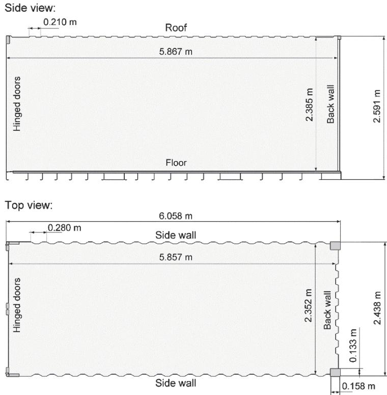
Figure 4: Dimensions of the container.
