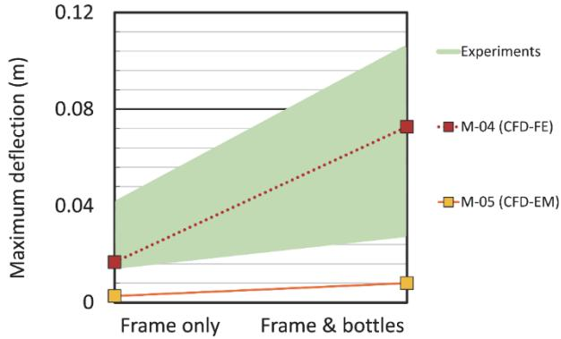
Figure 17: Comparison of model predictions for maximum deflection.
