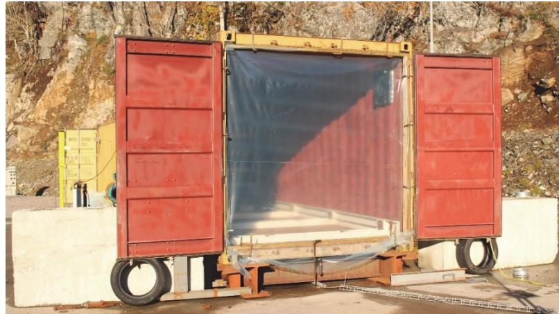
Figure 7: Container doors in fully open position, and opening covered by a polyethylene sheet.
