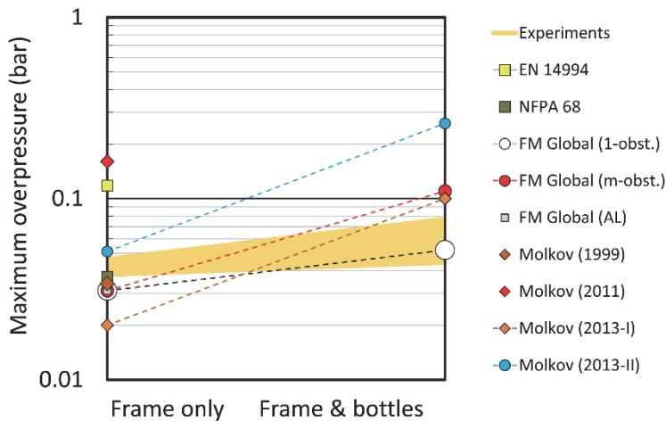
Figure 16: Comparison of model predictions for engineering models.
