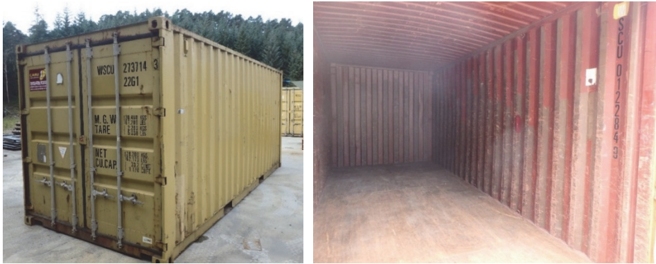
Figure 3: The 20-foot container (left) and the interior of the container (right).
