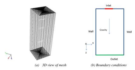
Figure 1. Mesh and boundary conditions used in the numerical simulation.
