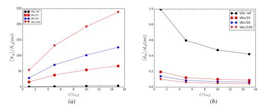
Figure 5. Number of aggregates normalized by initial number of aggregates (a) and diameter of aggregates normalized by initial diameter of aggregates (b) in function of fluid dissipation normalized by reference case. When the resistance of aggregates decreases and the fluid dissipation increase, the breakage of aggregates will be more important. The results show that the number of aggregates increases and whereas the mean diameter of aggregates decreases. The trend obtained was expected.
