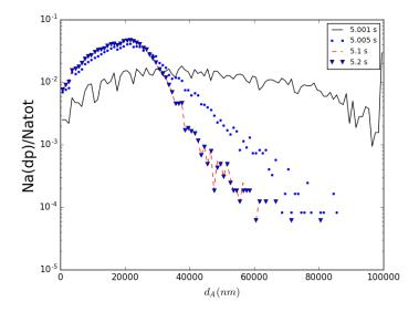
Figure 4. Distribution function of aggregate diameter for different times in the simulation within the whole domain When aggregates move away from the strong dissipation field, the breakage becomes weak and the particle size distribution does not change as showed in figure 4. For this case, the mean diameter of aggregates is still in the microscale. However, we can observe that there are 1% of aggregates in the first intervals which are in nano-scale.
