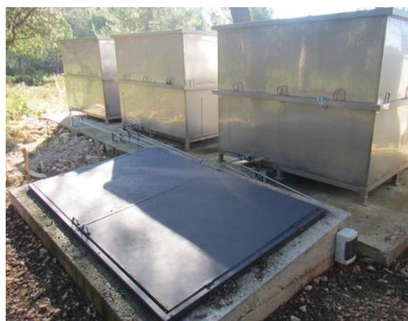
Figure 2: Three lysimeters and their percolate collecting system
