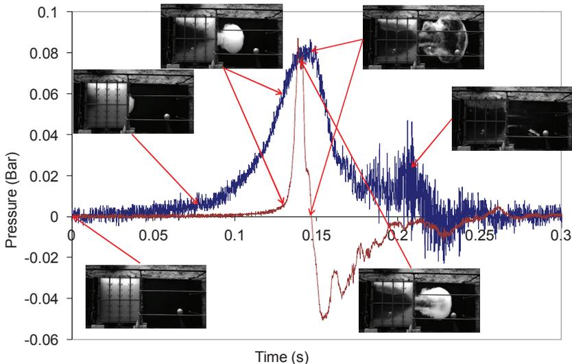
**Fig. 5:** Internal overpressure evolution, flame evolution and the external overpressure at 2 m (Test 6 : rear ignition, % H2 = 16.5, homogeneous, vent area 0.5 m<sup>2</sup>)
