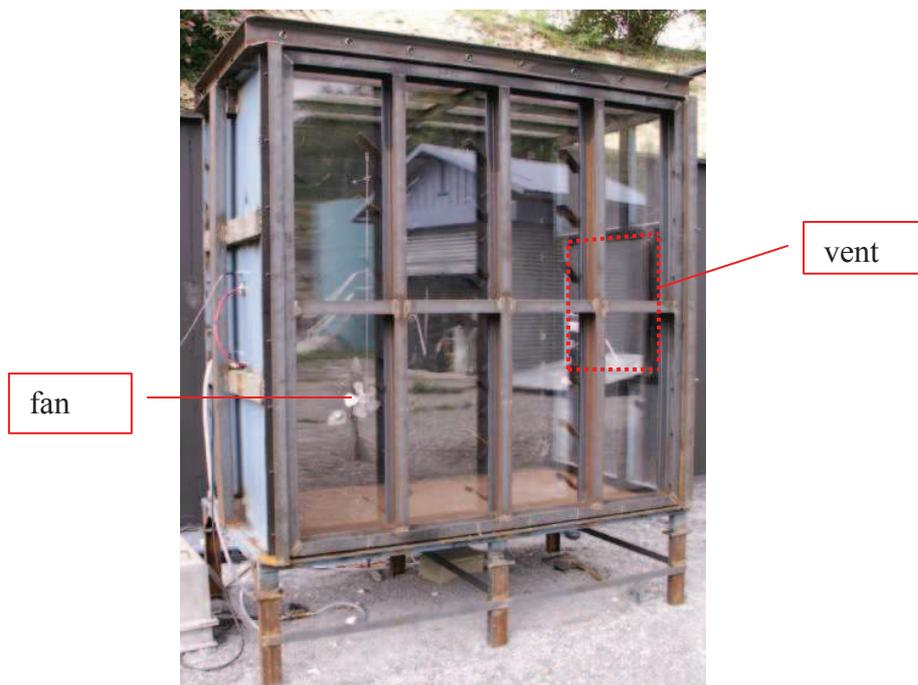
**Fig. 2:** The 4 m<sup>3</sup> chamber (2 m high, 2 m high, 1 m deep).
