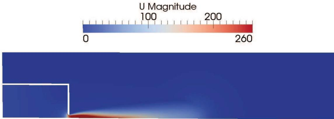
**Fig. 15:** Flow velocity in the 54 m<sup>3</sup> chamber at 210 ms (test 5)
