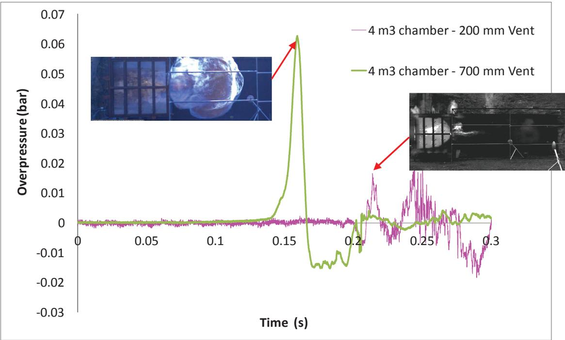
**Fig. 6:** Overpressures measured at 3 m from the vent for the external explosion developed from the 4 m<sup>3</sup> vessel only with the 700 mm vent (test 2- green curve) and the 200 mm vent (test 3 – pink curve)
