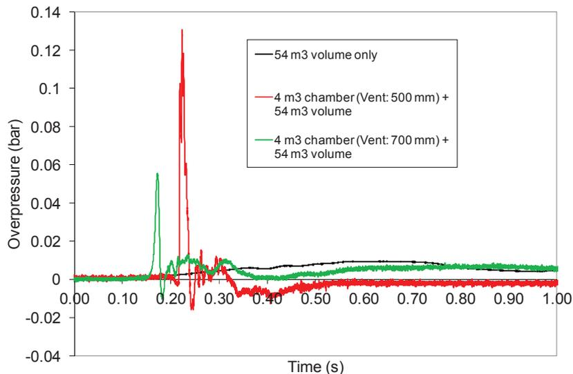
**Fig. 7:** Overpressure in 54 m<sup>3</sup> volume
