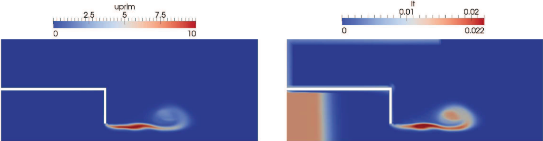
Fig. 14: Turbulent intensity U' (m/s) and turbulent length scale l_t (m) (test 2)
