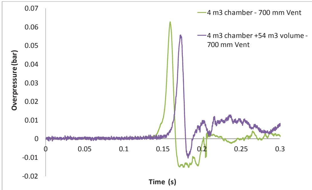
**Fig. 8:** Overpressures measured at 3 m from the vent for the external explosion developed from the 4 m<sup>3</sup> vessel only (test 2) and the explosion of 54 m<sup>3</sup> volume ignited by the 4 m<sup>3</sup> chamber explosion (test 4)
