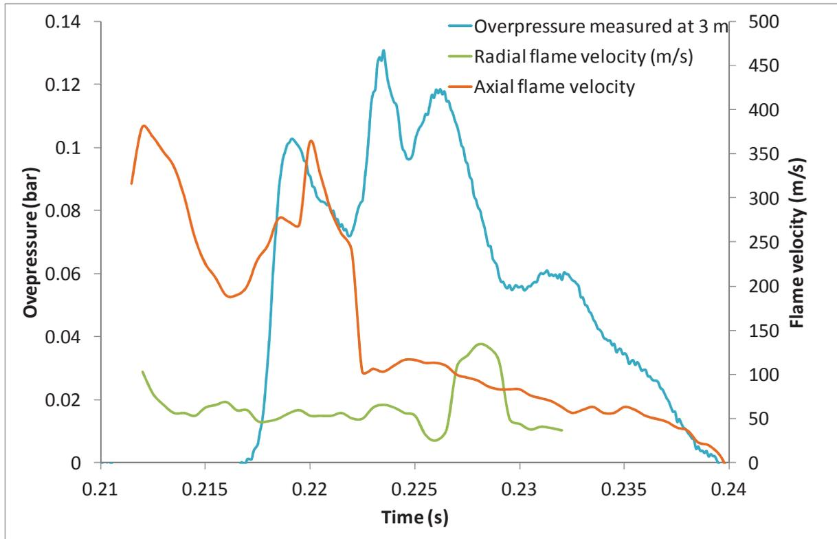
**Fig. 10:** Maximum flame velocity along the vent axis (orange curve) and perpendicular to the vent axis (green curve) and external overpressure (in the 54 m<sup>3</sup> volume)
