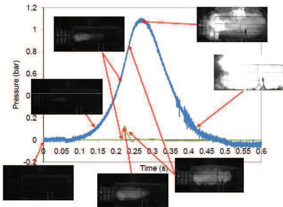
**Fig. 9:** Internal (blue curve) and external (green curve) overpressures. Test 5: 4 % C<sub>3</sub>H<sub>8</sub>-air mixture, homogeneous, rear ignition, 0.04 m<sup>2</sup> vent
