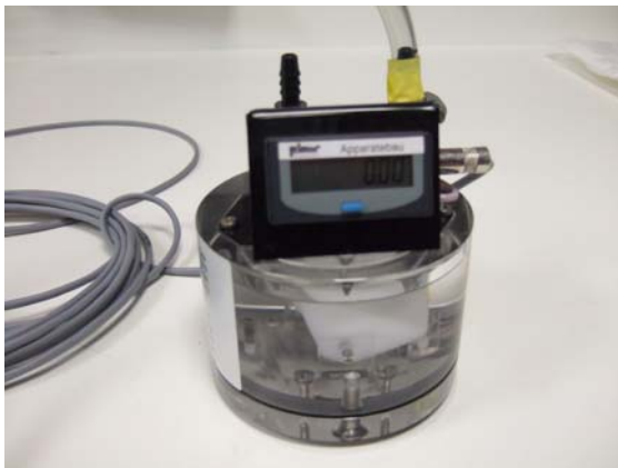
Figure 2: View of the automatic volumeter MGC-1 (PMMA cell) filled with Silox fluid.
