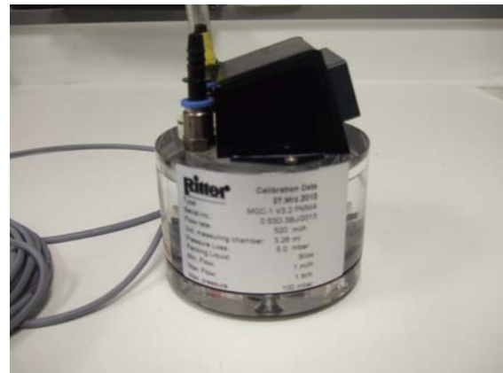
Figure 2: View of the automatic volumeter MGC-1 (PMMA cell) filled with Silox fluid.
