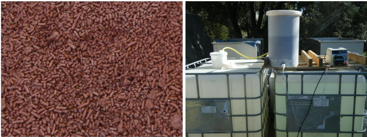
Figure 5: Granulated MBR, and water treatment at pilot scale
