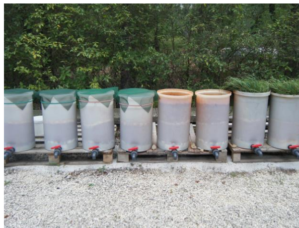
Figure 7: Lysimeters of spent MBR with different top layer
