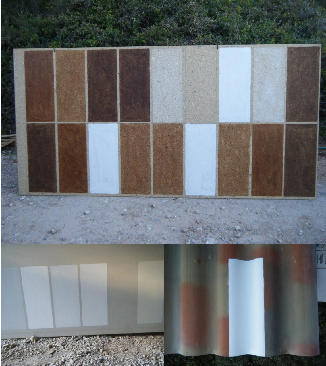
Figure 1 : Paints and varnished with ENPs additives, and paints containing ENPs on wood panel, plaster with cardboard, and cement plate
