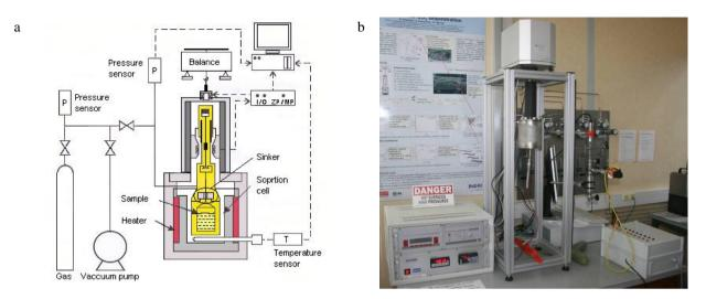
Fig. 1. Magnetic suspension balance: (a) diagram of the equipment; (b) photography of the equipment. Note that GC apparatus is not shown.
