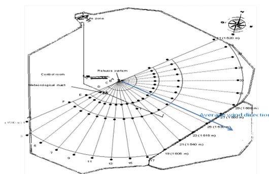
**Figure 10:** The whole measurement area in CEA-CESTA for the ammonia experimental test cases; sensor arcs locations (distances from the release system : 20 m, 50 m, 100 m, 200 m, 500 m, 800 m and 1700 m for corresponding referenced letters A, B, C , D, E, F, G)
