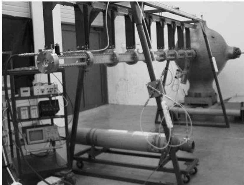
*Figure 1: equipment used by Kerampran (2001), 4 m long tube, 40 mm wide, square cross section*
