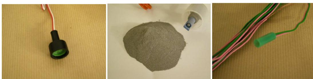
Figure 7 : Ignition devices. From left to right : 5000J electric igniter, flash powder, 60J pyrotechnical match
