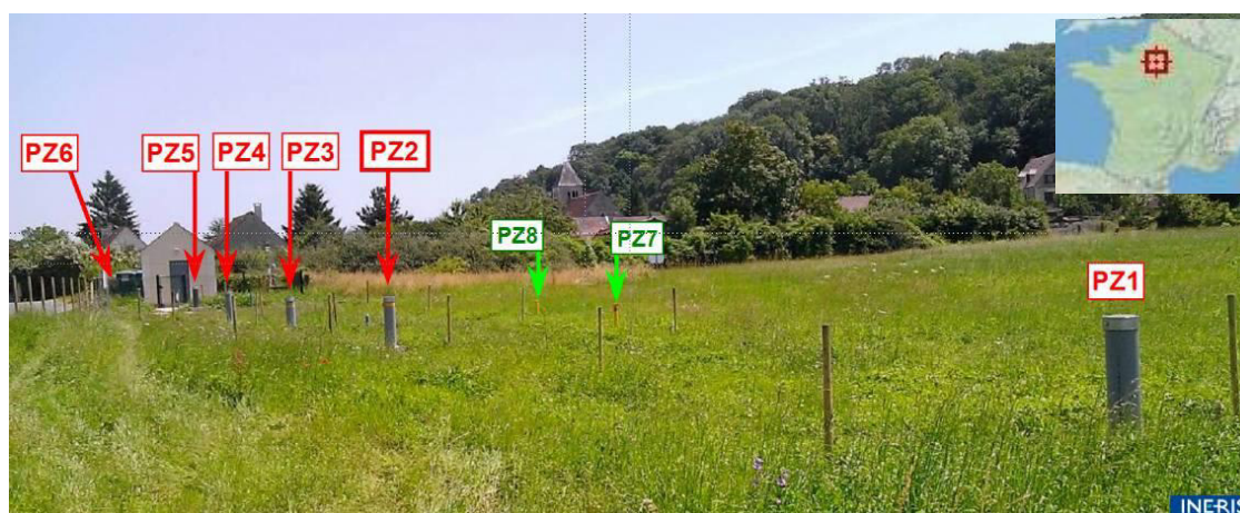
Fig. 1. The experimental site of Catenoy with its piezometers PZ1 to PZ8
