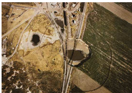
Fig 1 Land Subsidence in Central Kansas Related to Salt dissolution
