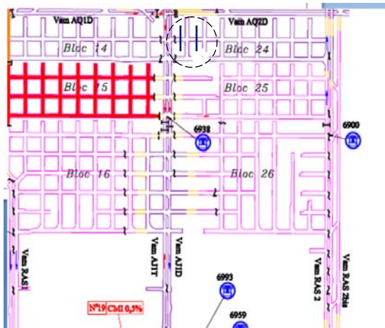
Figure 2: Section through Storage Area and location of cracks (blue) (MDPA, 2015) (Key: Bloc – Block).
