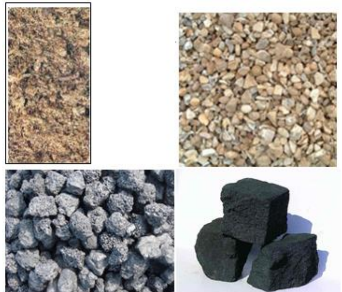
Figure 9. Example de peat, limestone and coke material for filling the trench.
