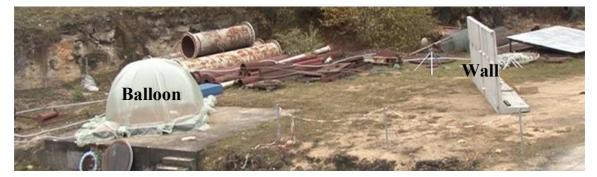
Figure 1: test platform with hemispherical balloon and protective wall of 6m length, 10 m between both
