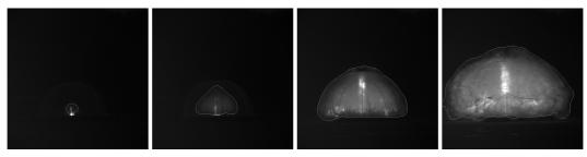
Figure 3: Processed images of the deflagration of the flammable mixture (10 ms between frames).
