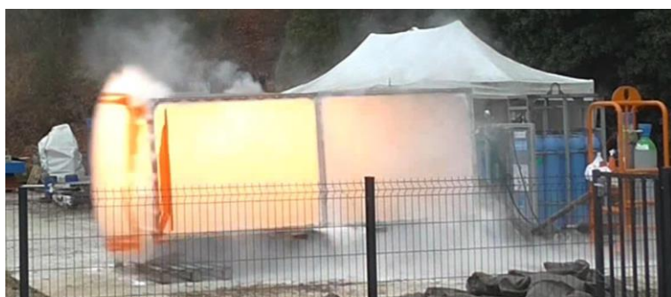
Figure 1. Explosion in a 10 m 3 vessel with a transparent face
