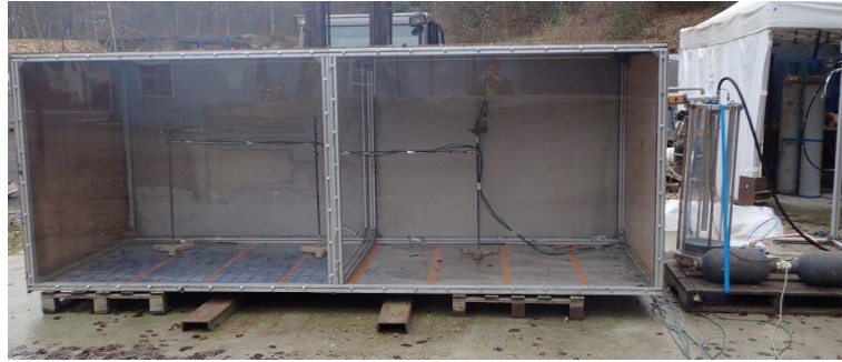
Figure 2. 10 m 3 vessel with a transparent face
