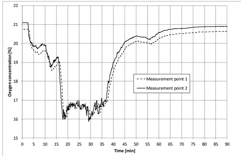
Figure 4: Evolution of oxygen concentration downstream the fire (car2).
