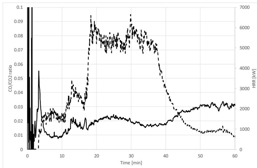
Figure 5: Evolution of CO/CO<sub>2</sub> ratio along time (continuous line) and HRR (dotted line) for car2.
