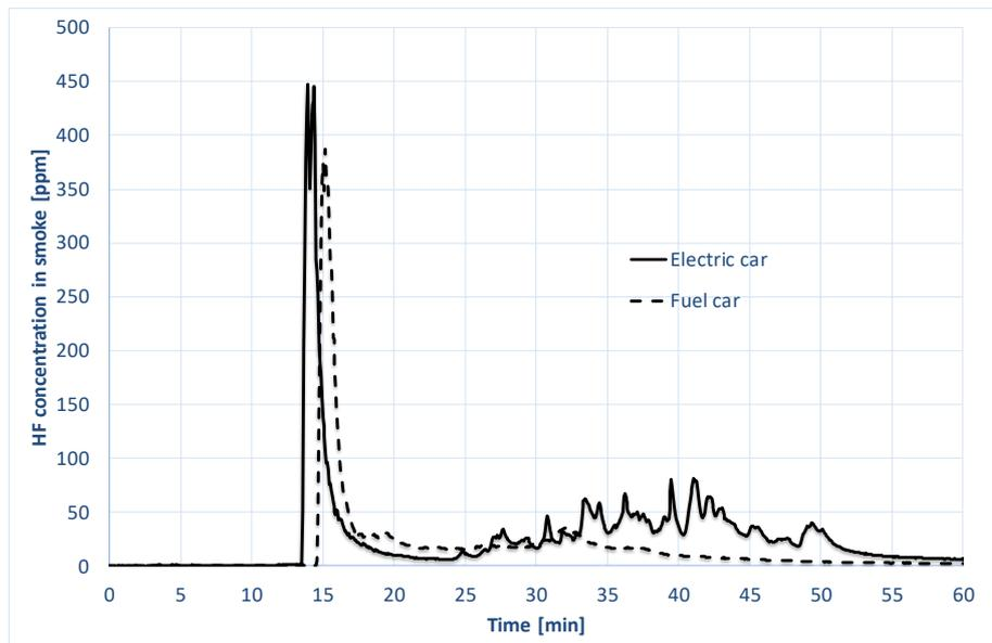
Figure 7: HF emission factor during the electric car (car 4) burning vs corresponding ICE car (car 2).
