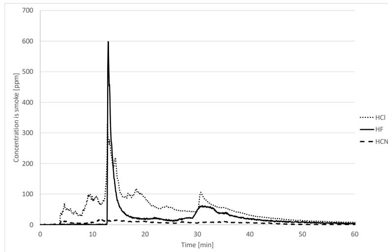
Figure 6: Acid gases concentration of acid gases in smoke versus time for car 3.
