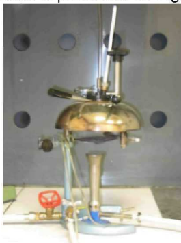
Figure 3: View of INERIS manual Pensky-Martens closed-cup flash point apparatus
