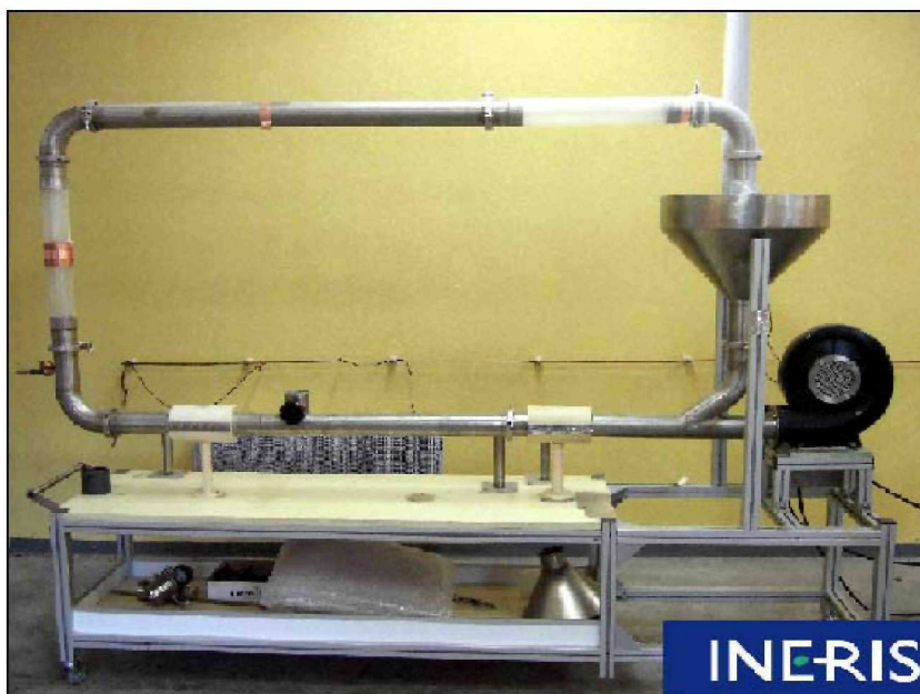
Pilot test bench for validating the measurement instruments
