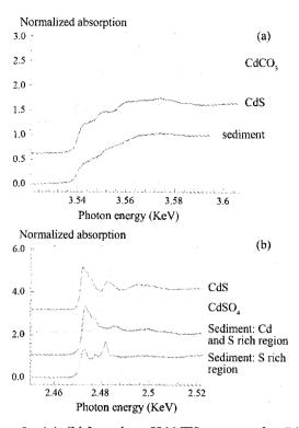
Figure 3. (a) Cd  $L_{II}$ -edge  $\mu$ XANES spectra of a Cd-rich region of sediment and reference compounds and (b) S K-edge  $\mu$ XANES spectra recorded on two sediment samples (one Cd and S rich region and one S rich region)
