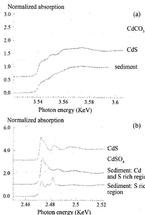
Figure 3. (a) Cd L<sub>III</sub>-edge  $\mu$ XANES spectra of a Cd-rich region of sediment and reference compounds and (b) S K-edge  $\mu$ XANES spectra recorded on two sediment samples (one Cd and S rich region and one S rich region)
