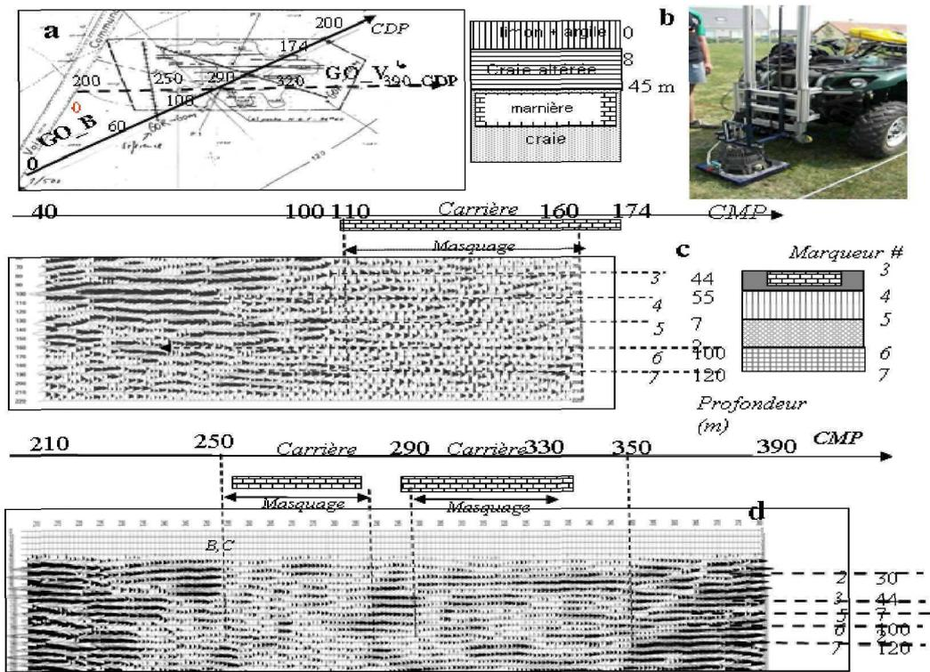
Fig.2.Site of Godeville a) positions of profiles et and void limits; b) P vibrator mounted on an all terrain vehicle (quad) c) Section GO\_B and interpretation d) Section GO\_V and interpretation.
