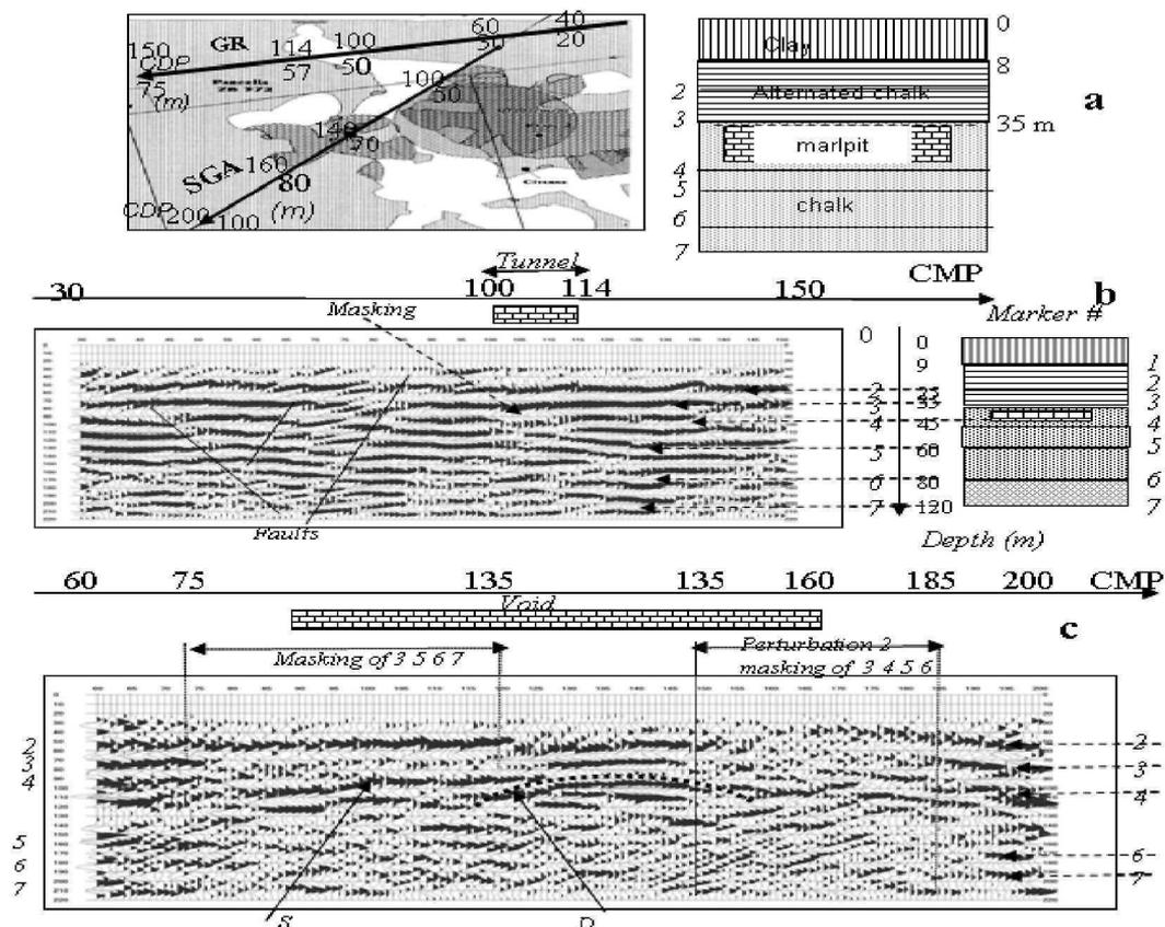
Fig.1. Site of St Gilles a) Location of profiles, the void limits and geological structure; b) Section GA and interpretation c) Section SGA and interpretation
