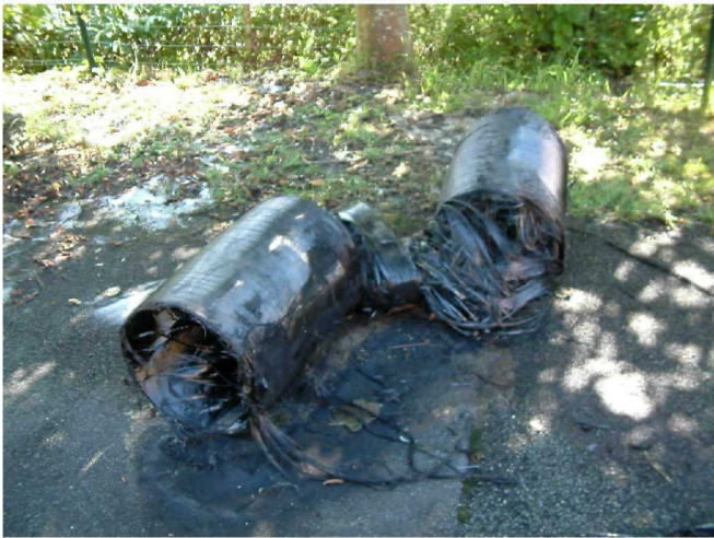
Figure 11: Tank n°1 after burst (Courtesy SDIS 25)
