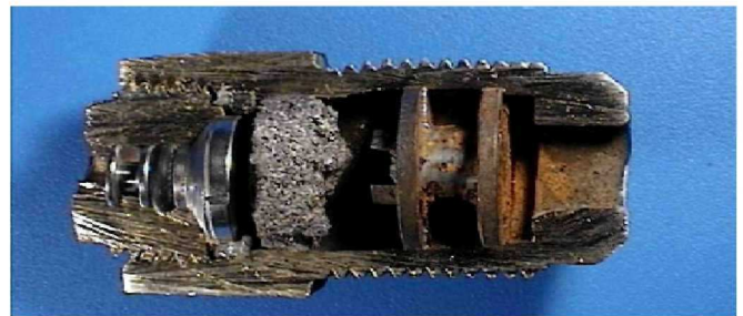
Figure 7: Example of one closed PRD from tank n°1. Picture shows that the metal fuse did not have time to melt completely (from [6])
