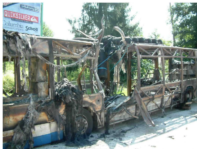
Figure 9: Side view of the bus with tank n°3 hanging (Courtesy SDIS 25)
