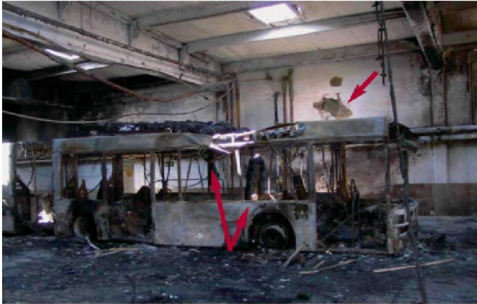
Figure 4: Destroyed bus with red arrows pointing (from right to left), tank n°3, hanging tank n°2 and hole through which tank n°1 flew (from [6])
