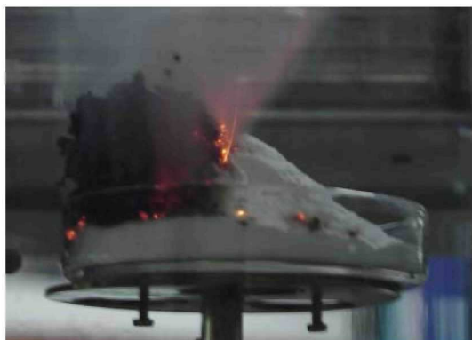
Figure 4: Smoke Powder 1 burning in the Tewarson apparatus operated by INERIS
