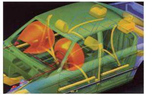
Figure 1: locations of pyrotechnics in a car (steering wheel, dashboard, doors, seat-belts...)
