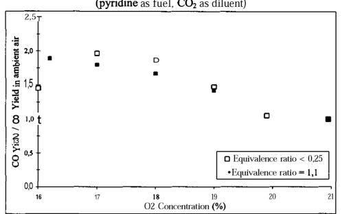
Figure 6: Ratio of CO yield to CO yield in ambient air as function of  $O_2$  concentration (pyridine as fuel,  $CO_2$  as diluent)
