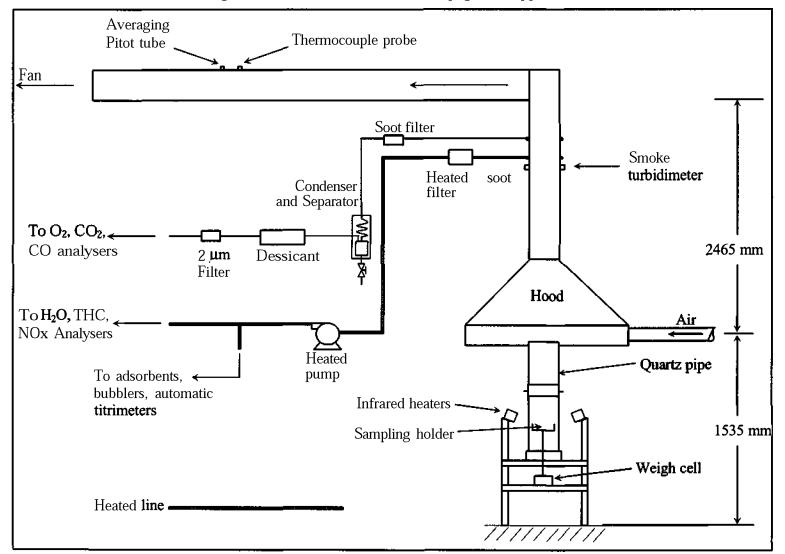
Figure 1 : Schematic of the Fire Propagation Apparatus
