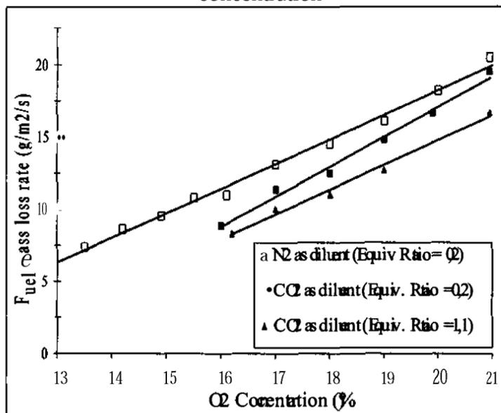
Figure 3: Normalised pyridine mass loss rate as function of O<sub>2</sub> concentration
