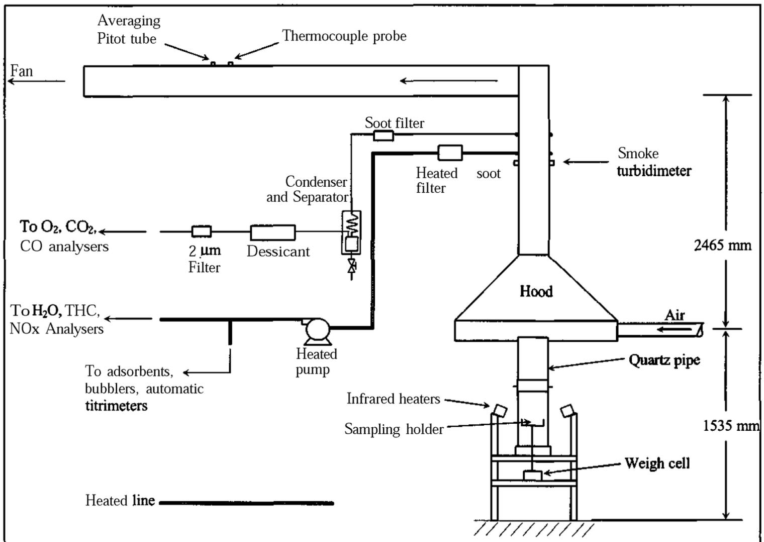
Two mass flow meters allow the operator to set the desired mass flow rate of air of up to  $300 \text{ Nl.min}^{-1}$ . Another mass flow meter allow the introduction of  $\text{CO}_2$ ,  $\text{N}_2$  or  $\text{O}_2$  into the incoming air for non-ambient combustion conditions. The air may thus be enriched or depleted in oxygen. The composition of oxidising stream is measured by an oxygen analyser, the sampling probe is located below the specimen holder in the combustion chamber.
