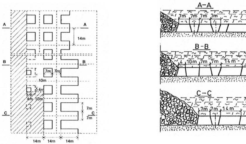
Figure 5: Examples of stages in the mining sequence
