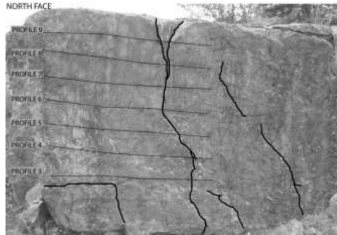
Figure 18: Depict of the North Face of the block in Chambéry (73). The black lines reveal the different discontinuities observed. The black horizontal lines identified each radar profile, profile 3 to 9 from the bottom to the top.
