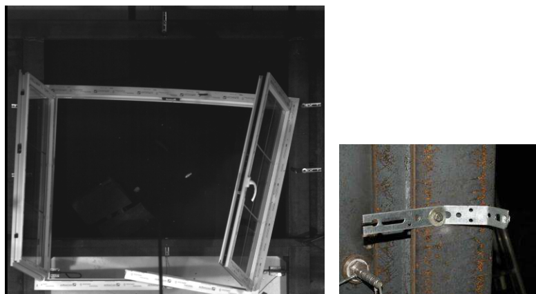
Figure 14: Response of window to blast wave (at left) - Angle bracket after the test (at right)
