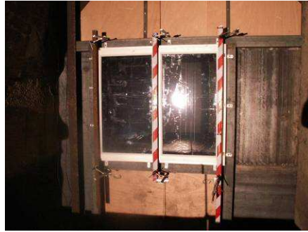
Figure 12: Annealed Insulating glass with wet-glazed security window film – Post test
