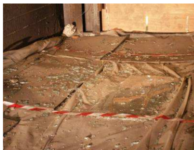
Figure 11: Annealed Insulating glass with daylight security window film – Post test
