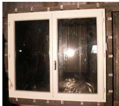
Figure 16: French style inwards opening window with reinforced locking system, laminated glass and reinforced anchorage system subjected to blast wave – Photography after blast test
