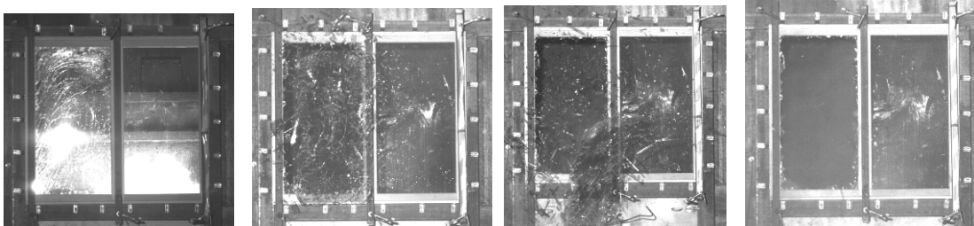
Figure 10: Annealed Insulating glass with daylight security window film subjected to blast wave
