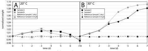
Fig. 3: Weight evolution of the samples in dry state at 20°C (A) and 30°C (B)
