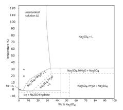
Fig. 1: Phase diagram of the Na2SO4-H2O system. Stars represent the concentration and Temperature for the two experiments.
