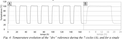
Fig. 4: Temperature evolution of the "dry" reference during the 7 cycles (A), and for a single cycle of 24 hours (B). The Temperature profile is in exp20.
