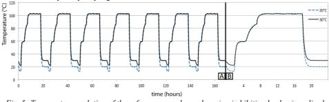
Fig. 5: Temperature evolution of the reference samples undergoing imbibition by demineralized water during the 7 cycles (A), and for a single cycle of 24 hours (B).
