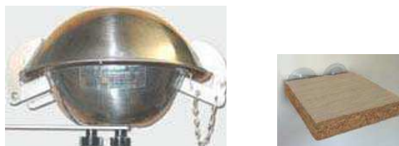
Figure 1. Passive air sampler and artificial desk surface used during the field campaign
