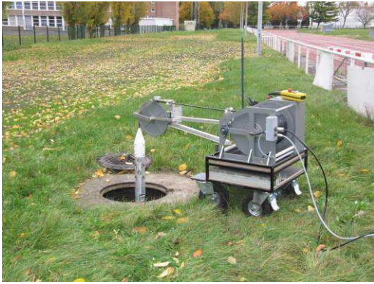
Photos 3 and 4: two examples of inspection of a shaft directly from the winder on its wheels
