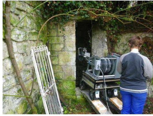
Photos 3 and 4: two examples of inspection of a shaft directly from the winder on its wheels
