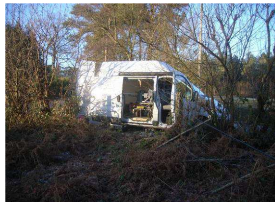
Photos 7 and 8 - Inspection of an inclined shaft through a 125 mm diameter borehole, the distance between the winder (in the van) and the tripod is about 80 m.
