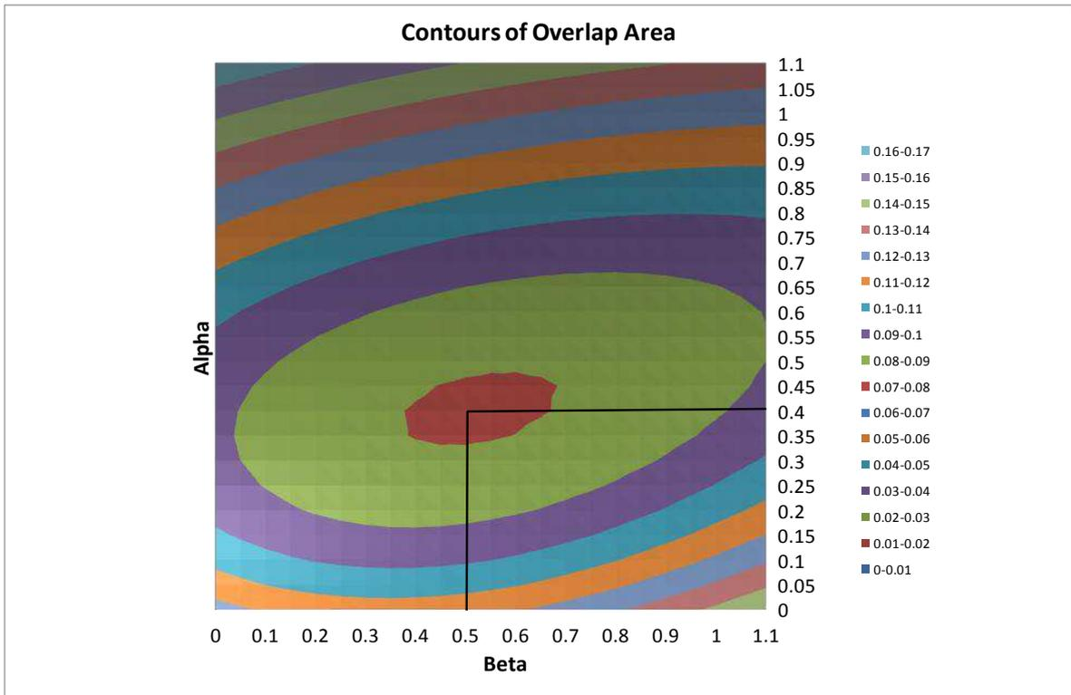
Figure 2: Values of the “overlap areas” of the distributions of safety coefficients for intact and failed pillars according to the values of  $\alpha$  and  $\beta$ .
