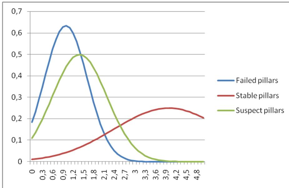
Figure 3: Probability density distributions of safety factors for the stable, suspect and failed pillars.
