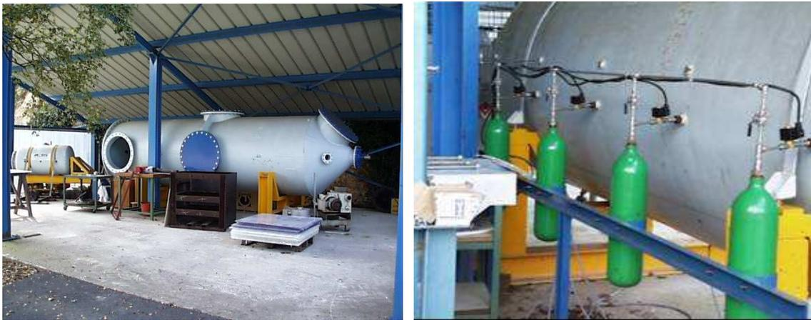
*Figure 2 : sketch (dimensions in mm) and views of the 10.5 m<sup>3</sup> chamber (injection device of the fuel on the right picture)*
