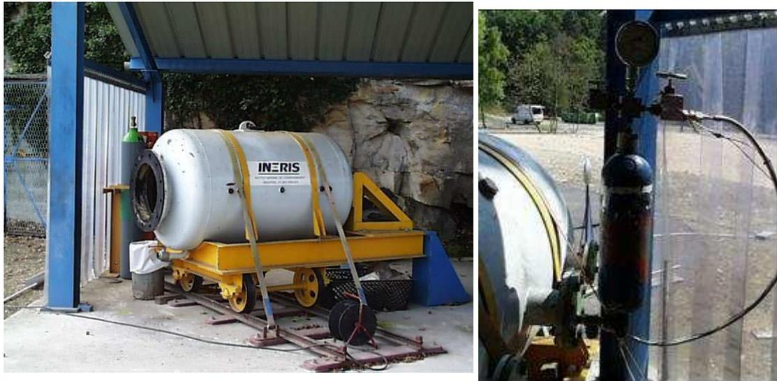
*Figure 1 : sketch (dimensions in mm) and views of the 1 m<sup>3</sup> vessel (injection device of the fuel on the right picture)*
