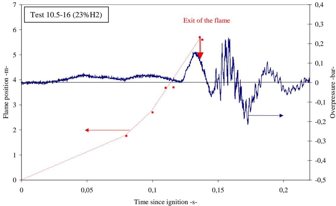
Figure 6 : Flame position, internal and external overpressures (10.5 m<sup>3</sup> vessel, rear ignition, 2 m<sup>2</sup> vent, % H<sub>2</sub> in air = 14; 23)
