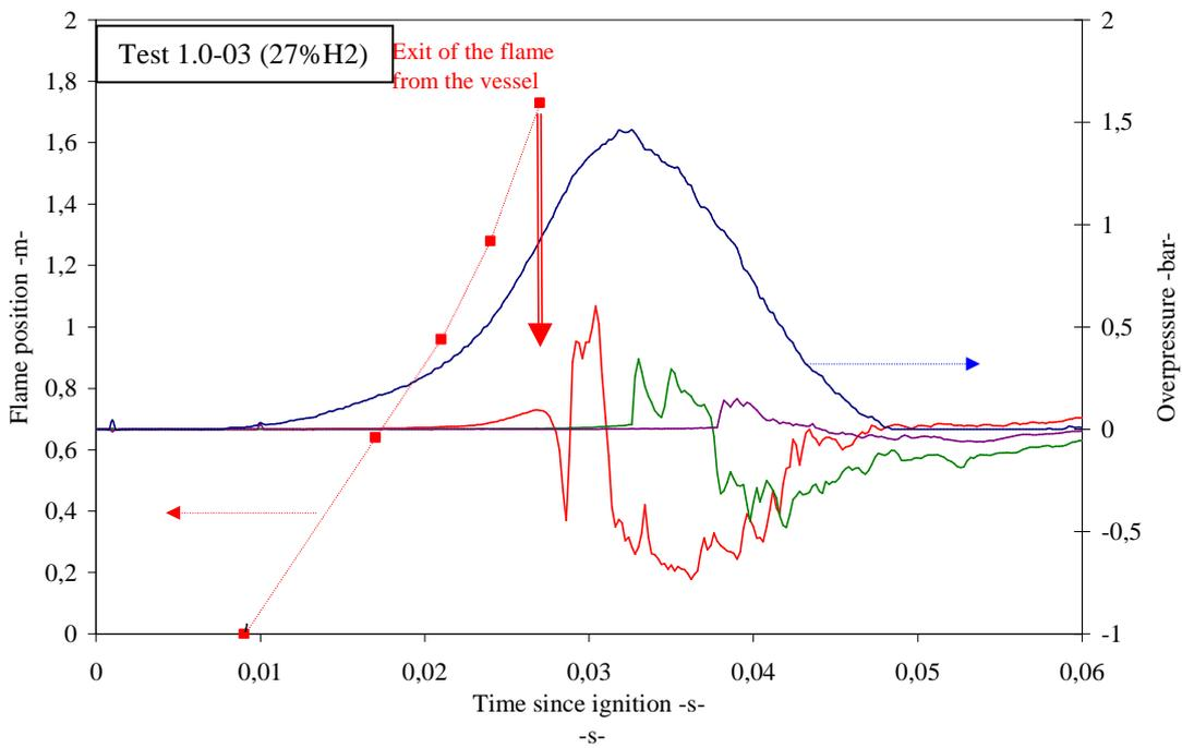
Figure 5 : Flame position, internal and external overpressures ( $1\text{ m}^3$  vessel, rear ignition,  $0.15\text{ m}^2$  vent, % H<sub>2</sub> in air = 10; 15; 20 and 27)
