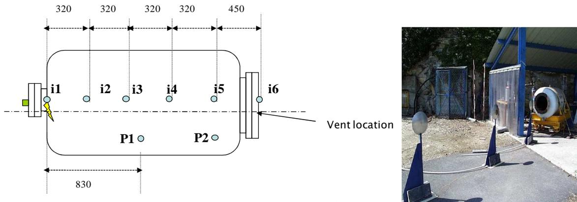
Figure 3 : instrumentation of the 1 m<sup>3</sup> vessel (inside and outside)
