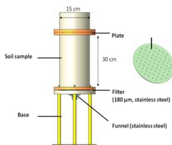
**Figure 1. Laboratory column**
