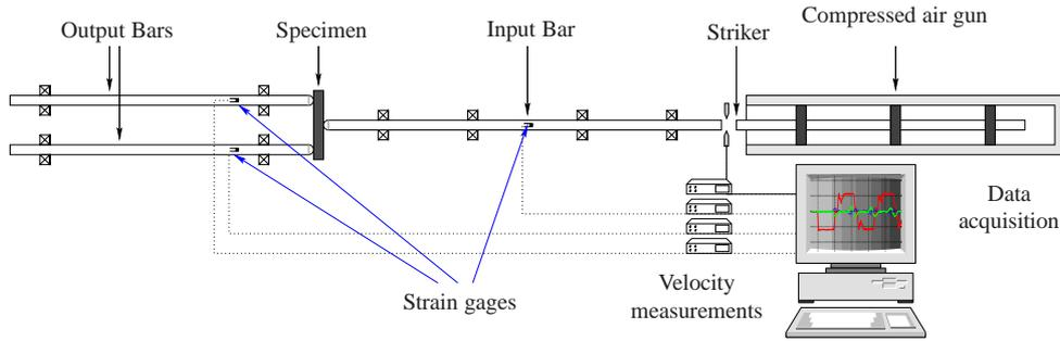
Figure 1: Schematic of bending test set-up and strain gages location
