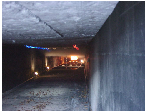
Fig. 11 Photography of the pool fire with the backlayering layer
