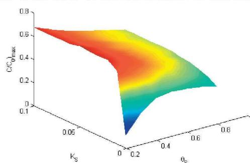
*Local variation of concentration versus time (left) and Variation of  $(C/Co)_{max}$  versus parameters  $K_s$  and  $\theta_s$ (right)*
