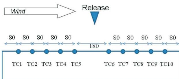
Figure 2: Thermocouples floating at the water surface
