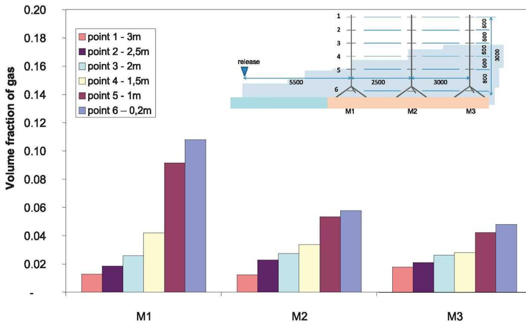
Figure 7: Calculated mean N<sub>2</sub> concentrations at the three atmospheric masts for trial No.7.
