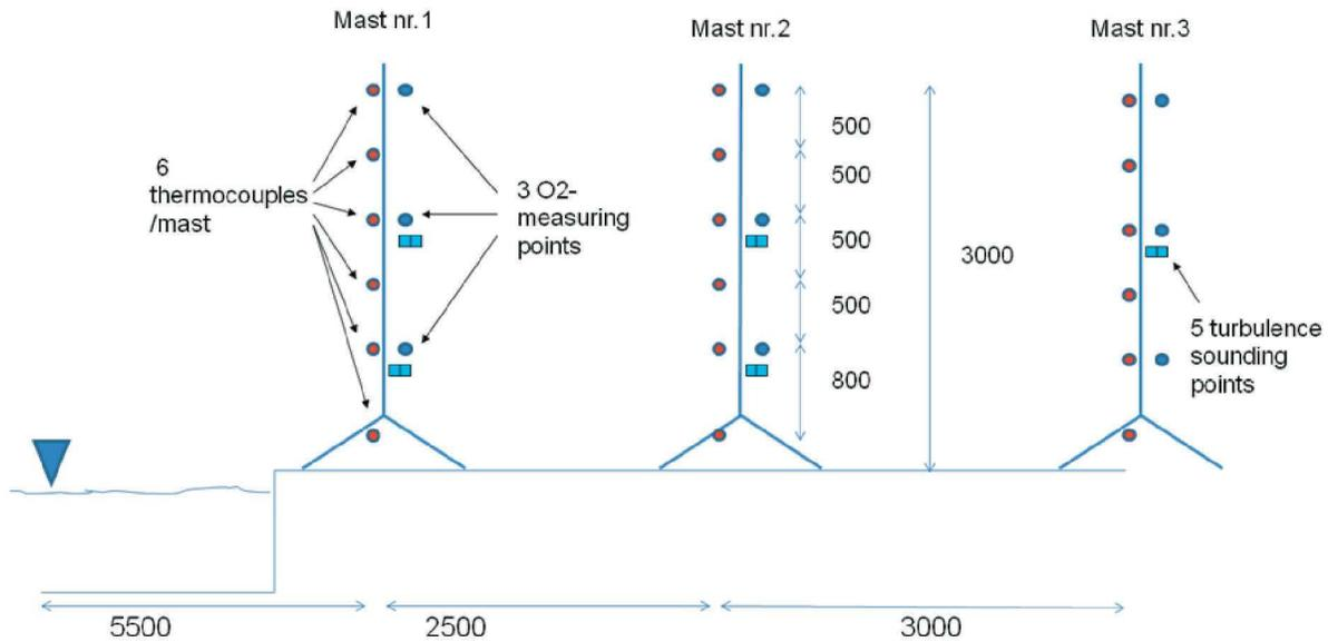
Figure 3: Atmospheric measurement equipment – Nitrogen is measured by means of a sampling device connected to an O<sub>2</sub>-analyser
