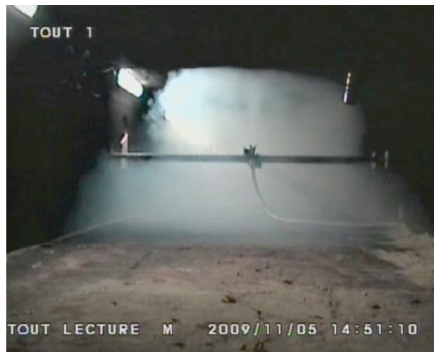
Figure 6: Photography of gas dispersion. Jet to the ceiling case, experimental case number 3.
