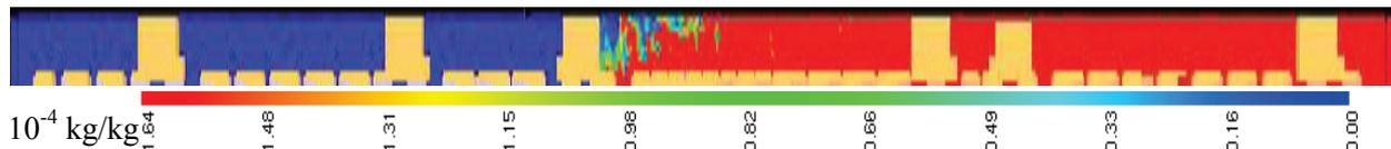
Figure 13: Acrolein dispersion in real scale tunnel considering a 3 m/s ventilation velocity. The maximum value that is represented is the toxic threshold for 10 minute exposure (73 ppm (mol fraction) = 1.4e-4 kg/kg (mass fraction)).
