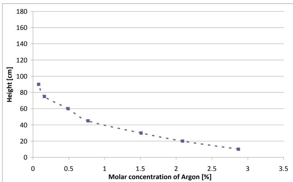
Figure 3: Vertical distribution of Argon concentration 15 m downstream the leak.
