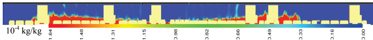
Figure 14: Acrolein dispersion in real scale tunnel without ventilation. The maximum value that is represented is the toxic threshold for 10 minute exposure (73 ppm (mol fraction) = 1.4e-4 kg/kg (mass fraction)).
