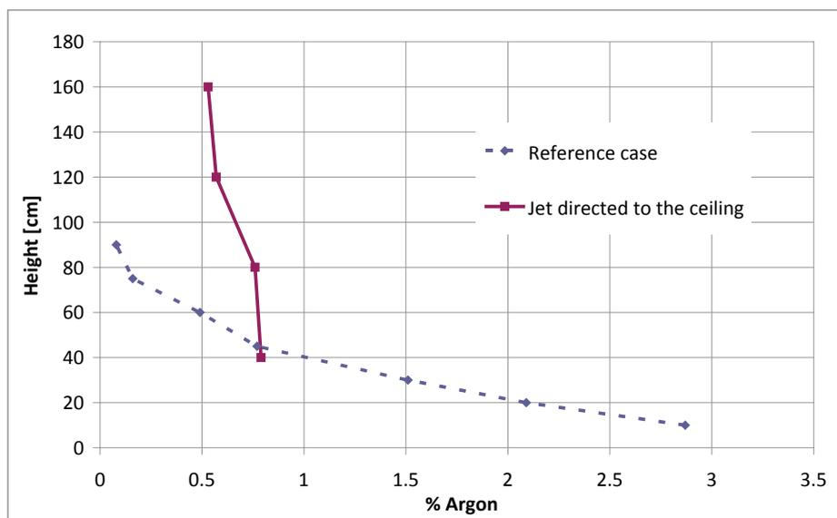
Figure 5: Vertical distribution of Argon concentration 15 m downstream the leak.
